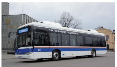
cold winters day. The biogas heating system allows all of the battery capacity to be used for driving the bus, which will improve the range significantly. On December 1<sup>st</sup> specially invited politicians, press representatives and the Swedish partners of the BBB extension stage project joined a short test trip and press event in Västerås.
