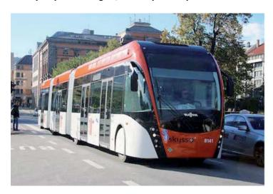
Bergen a 24-meter articulated biogas-electric serial hybrid from Belgian manufacturer Van Hool arrived on a freight ship on October 17<sup>th</sup>. A group of specially invited politicians and press representatives where at the Bergen harbor to greet the newcomer, which uses electric traction and a biogas engine to supply extra energy via a generator. On November 21st, the Norwegian partners of the BBB project organized an event with the new bus. All other partners
